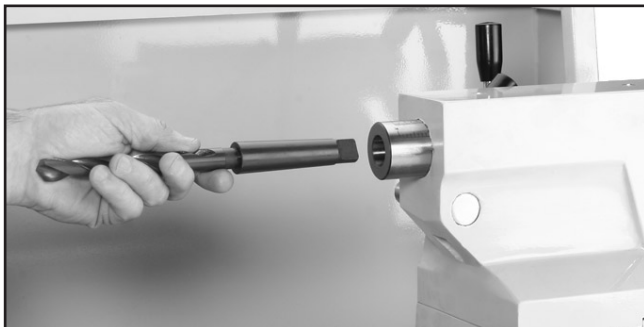
Figure 29. Example of drill bit installation.
